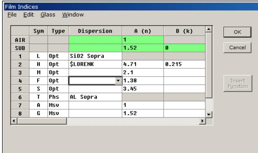
In reviewing how the BBAR problem was set up, we start with the Film Indices editor. Click **Setup...Film Indices <Ctrl+I>** to obtain the dialog box illustrated above. Several FilmStar screens, particularly those with data entry grids, can be resized by dragging edges or by choices in **Window**.
