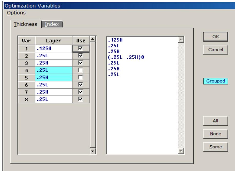
The program assigns variables as follows: If the design does not include parentheses the thickness variable is the layer number (from the substrate). If there are parentheses the variable is the layer number ignoring parentheses:
