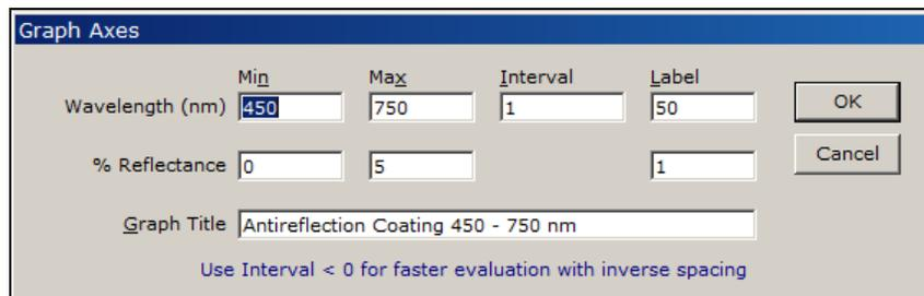
Click **Setup...Graph Axes <Ctrl+G>** for the Graph Axes editor. Edit fields as shown and click **OK**. Graph axes are automatically redrawn.
