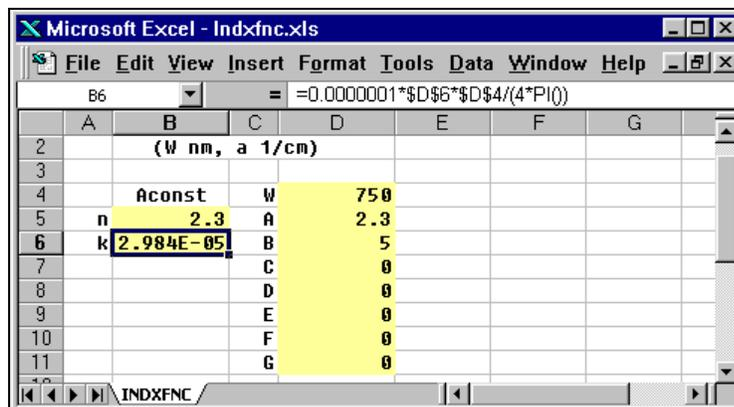
Consider an example using Microsoft Excel worksheet "indxfunc.xls". User-function **Aconst** returns n,k for a given absorption coefficient a (alpha) in 1/cm:  $k=1.e-7*a*W/(4*PI)$  for wavelength W in nanometers
