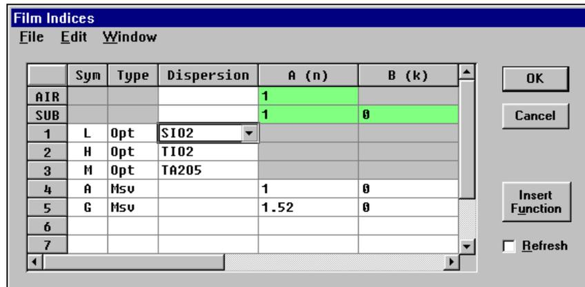
As shown in the above screen image,  $n=1$  for AIR and SUB is usually entered in the Film Indices editor. By defining "A" as a massive layer with  $n=1.0$ , we can insert an air gap.
