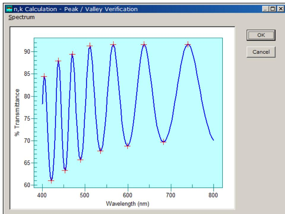
The entire data file is used in the calculation. If actual data shows spurious noise peaks, it is likely that the wavelength interval in the data file is too small. Data can be acquired again or Excel can be used to remove points. Click **OK** to proceed or **Cancel** if the data appears incorrect.
