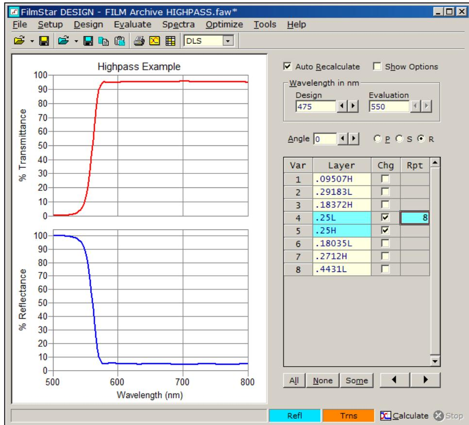
Click *Show Options* to enable a properties dialog below the layers grid. A scrollbar enables you to access the dialog without enlarging the DESIGN window. Interactor Mode *Design* supports up to 3 plots in the same graph while *Compare* lets you import a measured spectrum for reverse engineering.
