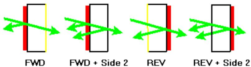
**Mode 5...**This special mode is intended for inverse synthesis. The uncoated surface is included in transmission but ignored in reflection. This corresponds to the practice of grinding the second surface in order to obtain more accurate reflection measurements.
